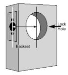
Holes - The diameter of the holes drilled through the door face to accommodate the existing, knob, lever, handle set or deadbolt.
